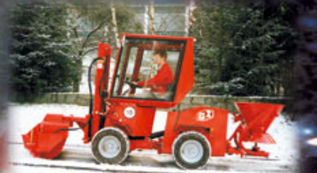
Snow Sweeping machine and granulation spreader
