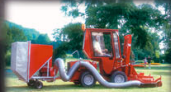
Front mower with vacuum system for grass and leaves
