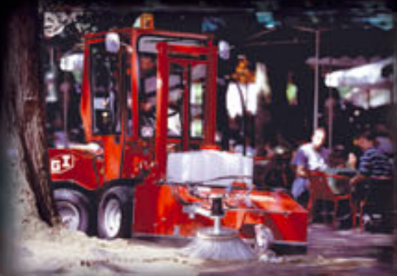
Sweeping machine with waste collector
