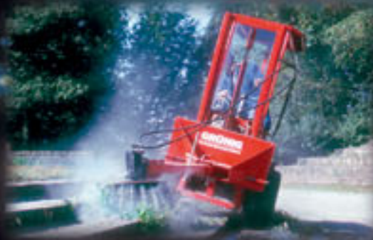
Hydraulic broom for weed removal
