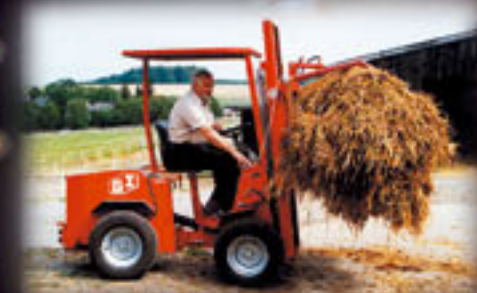
Hydraulic clamp for silage and hay
