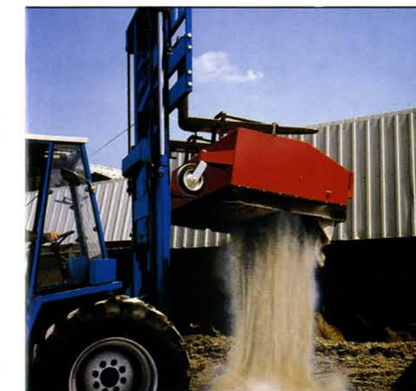
Emptying of the debris container with remote operation from the carrier vehicle directly into containers. (GSX-series)
